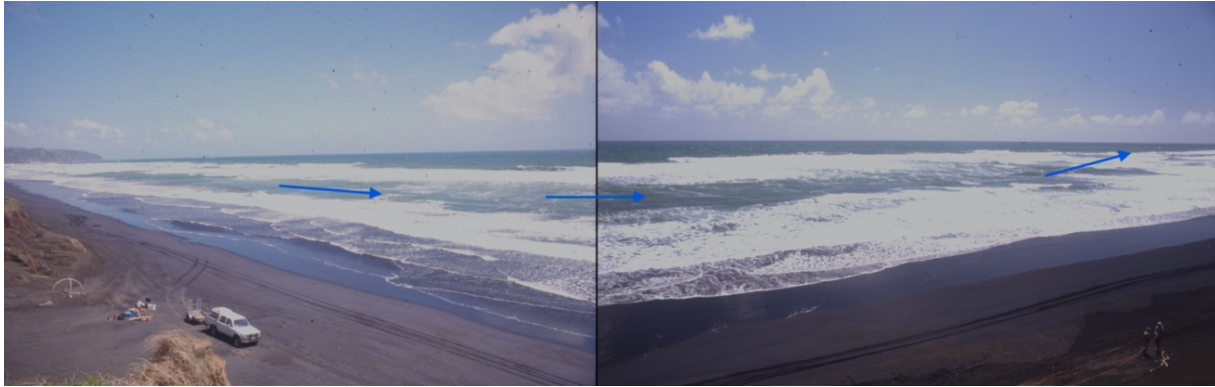
Figure 6. Surveying the rip current came with challenges. The extent of the feeder (blue arrows) is evident in the left image and the rip-neck almost imperceptibly flows obliquely offshore in the right image. (Photos: R.W. Brander.)
