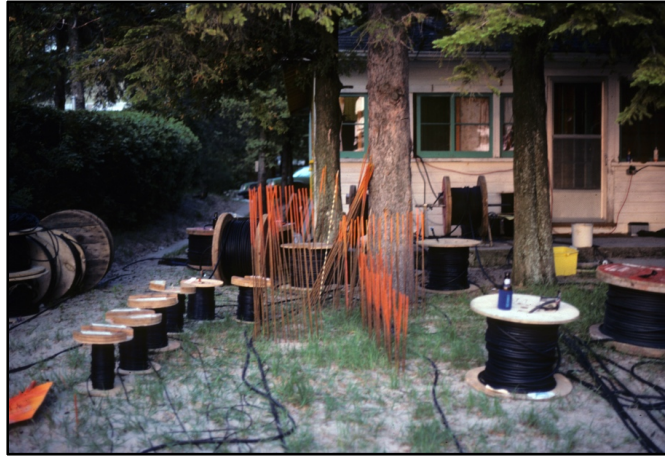
Figure 3. Spools of cable leading from submerged instruments to a data acquisition system in the accommodation cottage. In the center of the photo are dozens of Depth of Disturbance (DOD) rods painted with fluorescent dye for greater visibility in water. (Photo: B.O. Bauer.)
