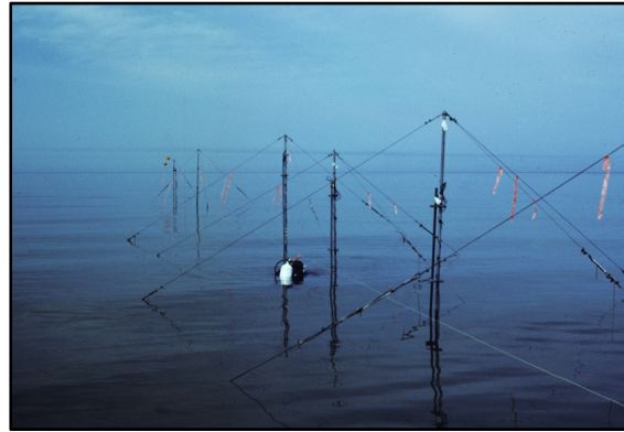
Figure 1. Resistance-type wave staff array deployed at Wymbolwood Beach, Georgian Bay, Ontario (1985). (Photo: B.O. Bauer.)
